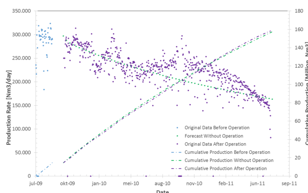
Figure 5.15: Second exception. Production is on the same level as it was before the treatment
