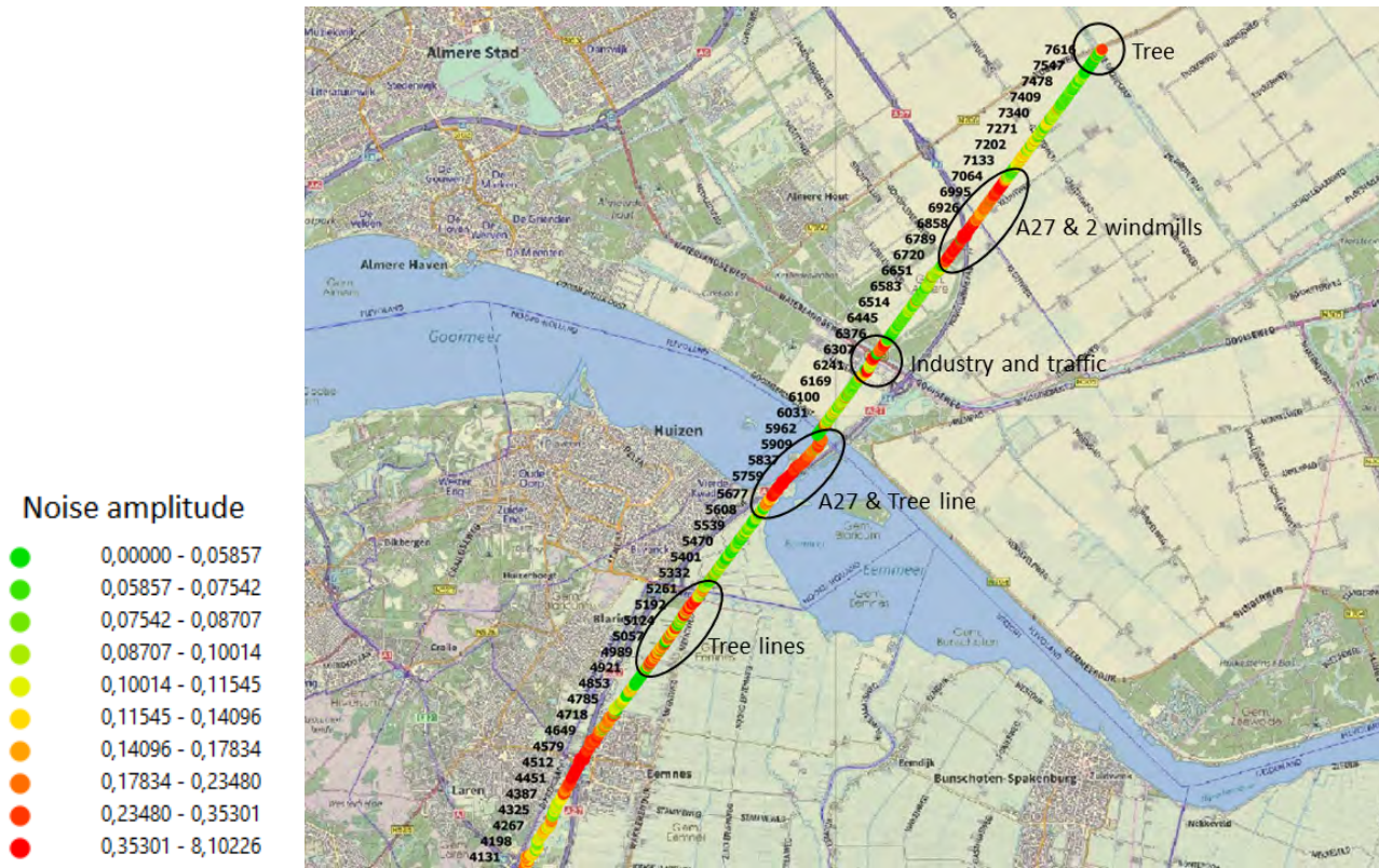
Figure 32: Map-view (1:65000) of noise amplitudes in the receiver domain of the northern half of test line.
