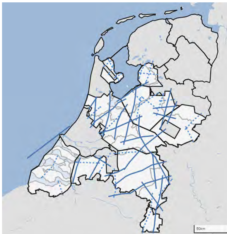
Figure 3: The planning for the SCAN 2D seismic acquisition. A solid line represents a seismic line that is either planned, currently being shot or finalized. A dashed line represents an optional survey extension. Source: http://www.scanaardwarmte.nl
