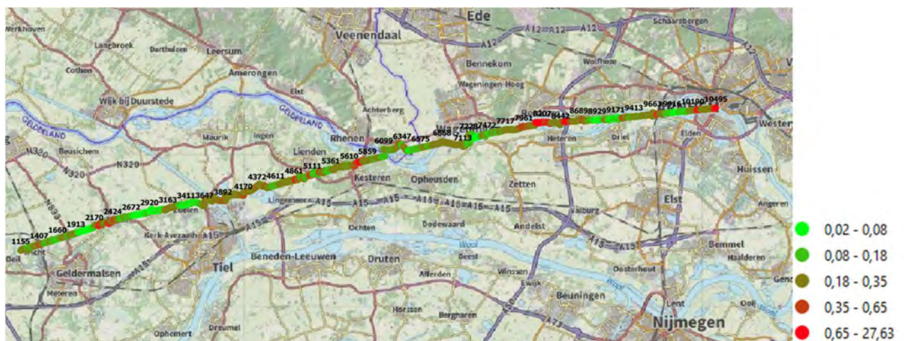
Figure 27: Map view of the average RMS noise amplitudes per receiver station for SCAN003. Numbers indicate receiver stations.
