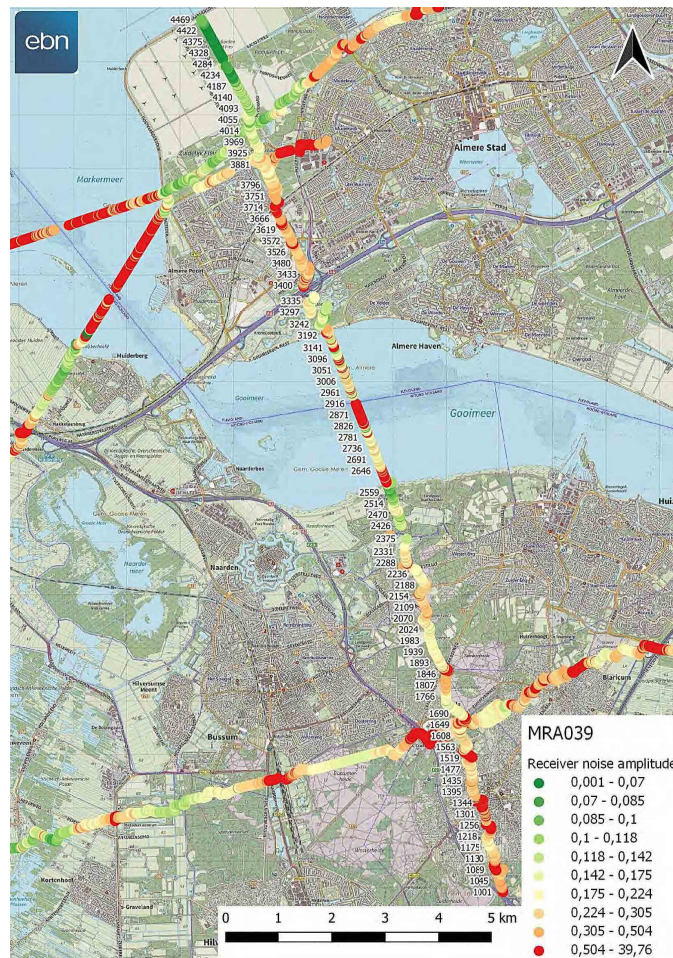
Figure 3.1.5.11: The noise per receiver visualized along the line. The color scale is based on the data of all the receiver data, showing noise relative to the other data points.
