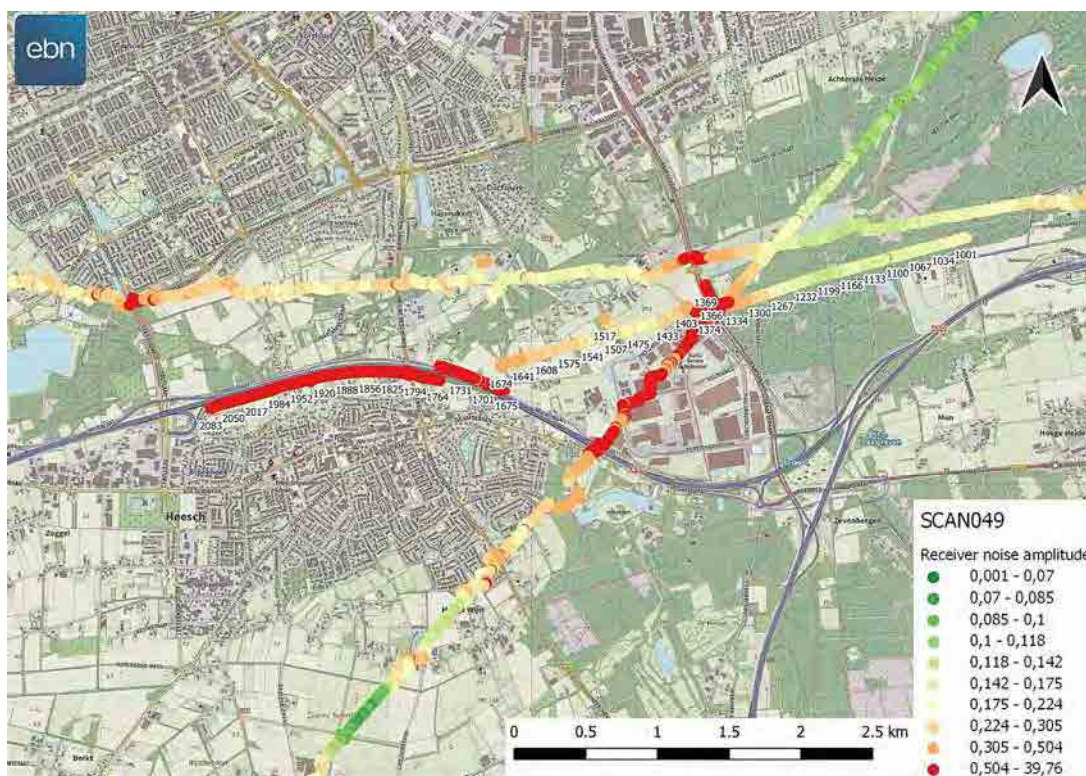
Figure 3.1.10.11: The noise per receiver visualized along the line. The color scale is based on the data of all the receiver data, showing noise relative to the other data points. Note that the station numbering is from right to left, unlike the other lines.
