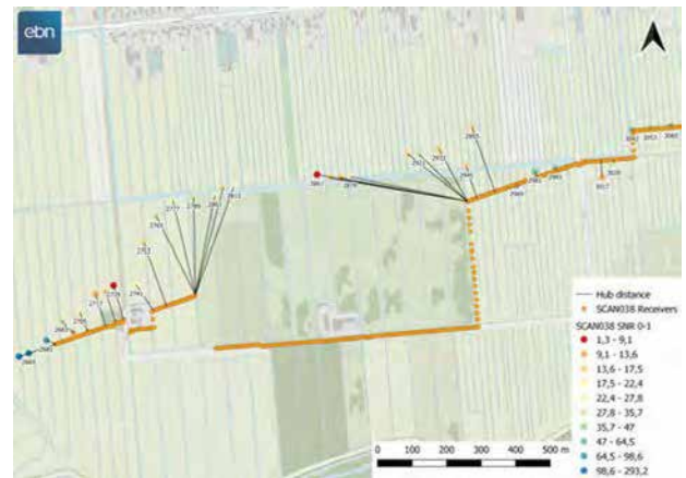
Figure 4.1.0.1: The non-uniform set up of the receivers and shots in the field on line MRA038.
